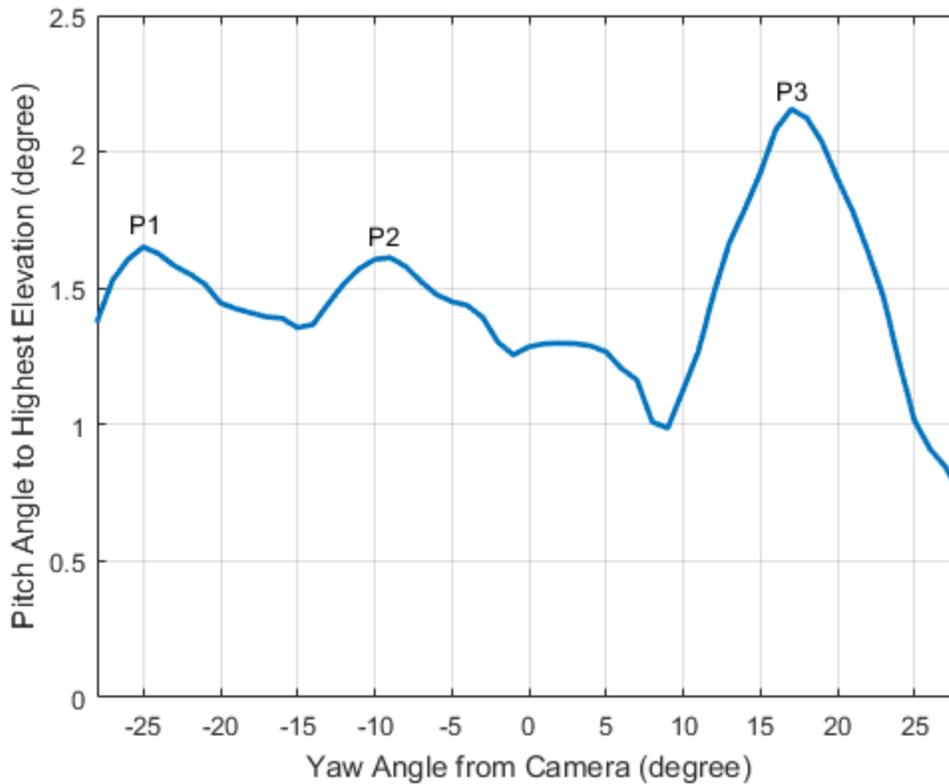
**Figure 4. Pitch Angle from Camera to Terrain vs. Yaw Angle from the Camera**
